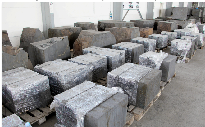
Figure 3. Blocks of mined ore cut into 50kg electrodes for feeding exfoliation cells, pilot test facility Rudolstadt.
