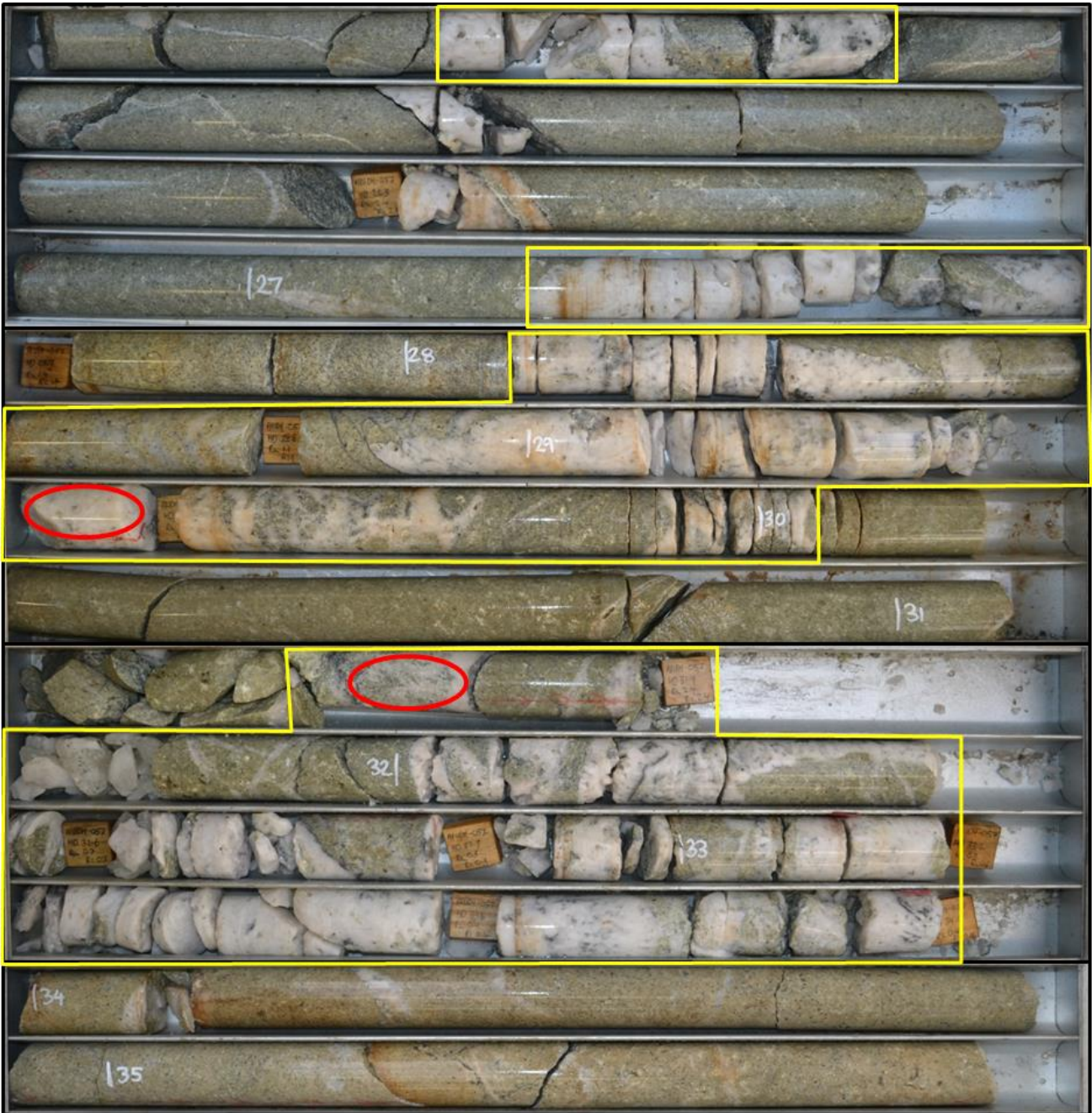
Figure 8. Diamond Drill Core from Hole A1UDH-057 24m to 35m. Visible Gold occurrences (Red Circles) within Dilational Breccia Zones (Yellow Boxes). Down-Hole depth (m) marked on Core.
