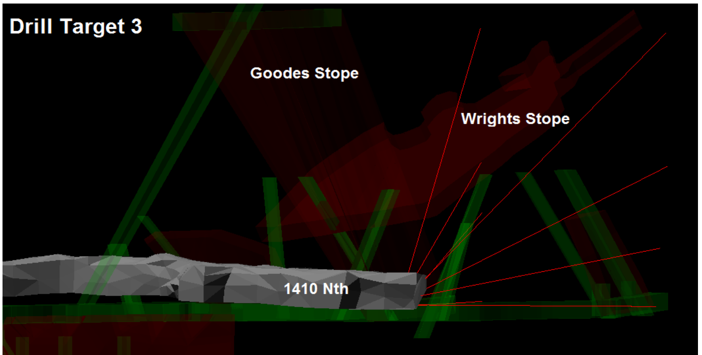
Figure 10. Isometric View of 1410 North Drive (looking East) showing Drill Target 3 planned holes.
