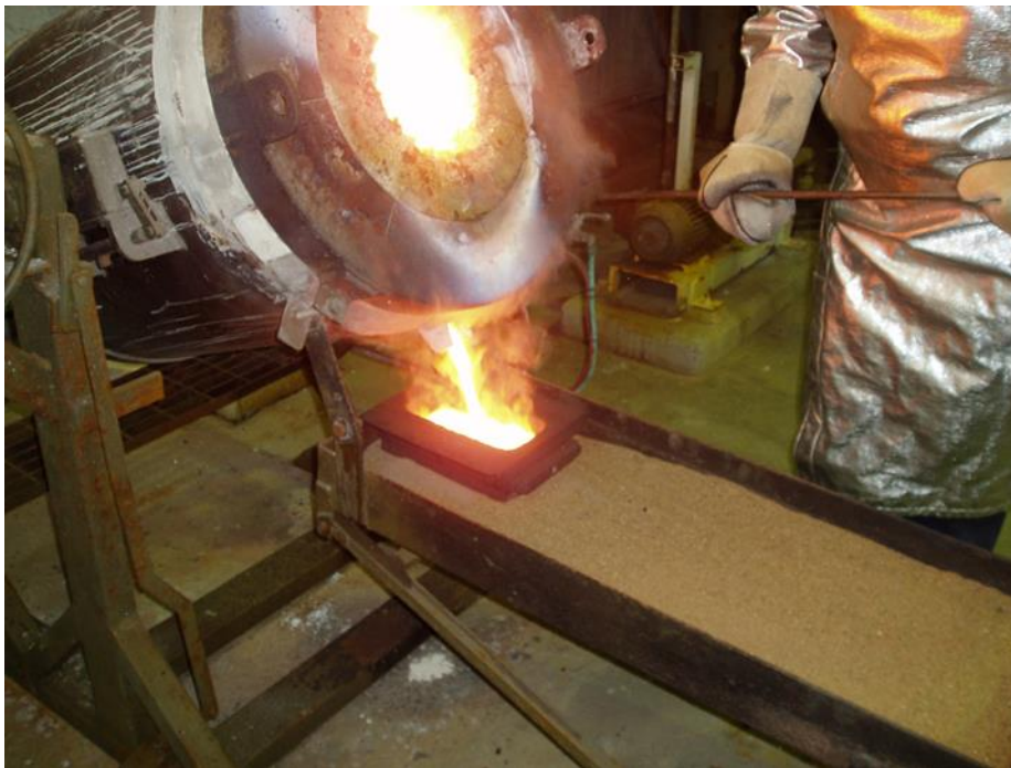
Figure 3. Gold Pour at Maldon Treatment Plant
