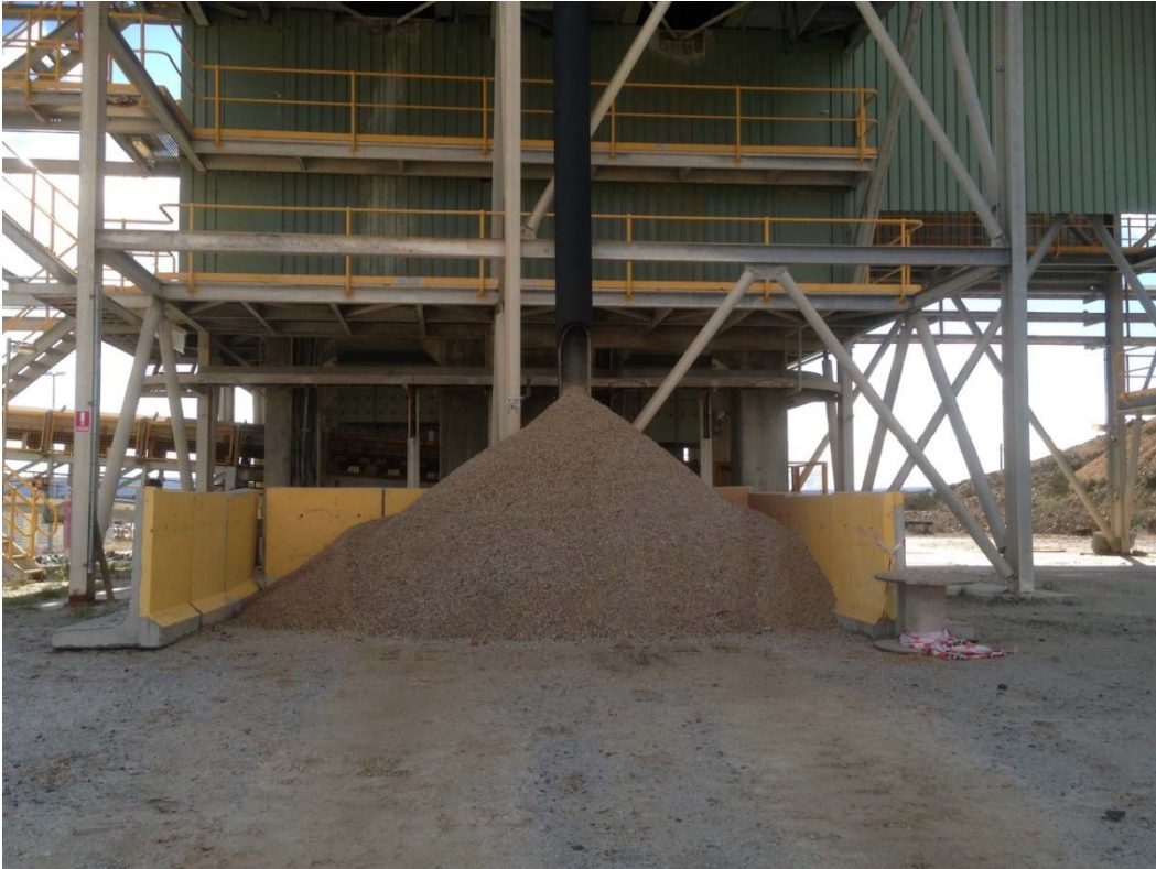
Fig 3: Stockpiling of feed for DMS circuit after tantalum removal
