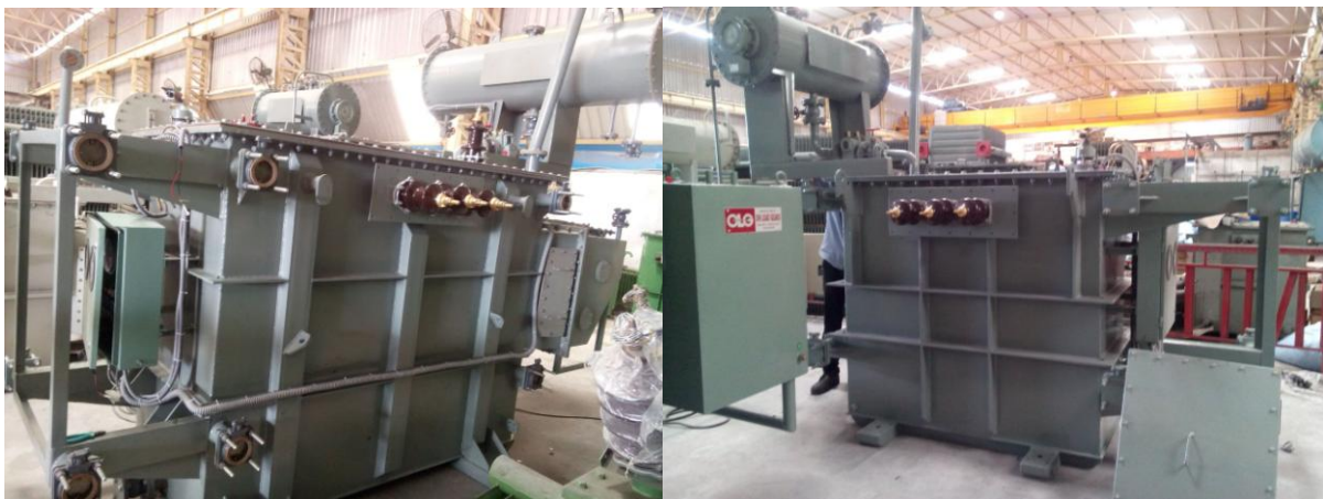
2.5 And 5 MVA Transformers
