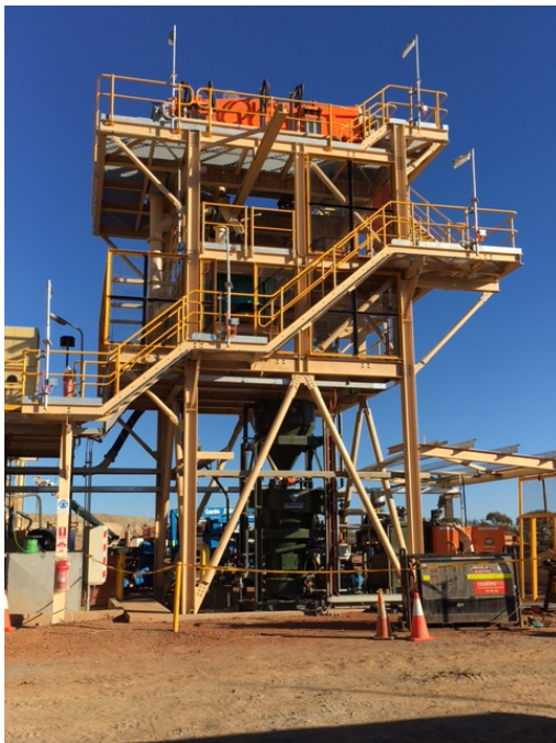
Figure 7 – Thunderbox mill - Gravity circuit installation
