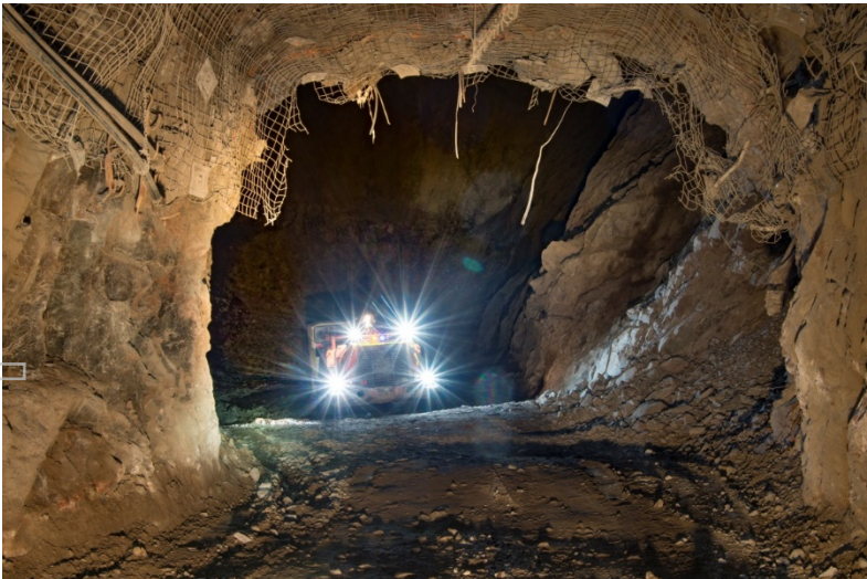
Figure 5 – Karari Underground – Bogging ore from the Dhoni 2140 stope
