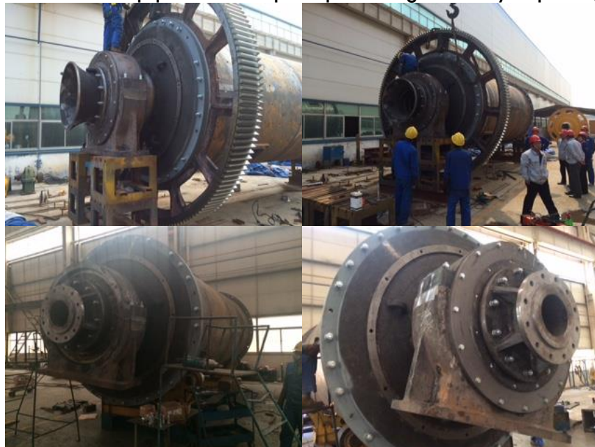
Ball mill equipment in final stages of fabrication
