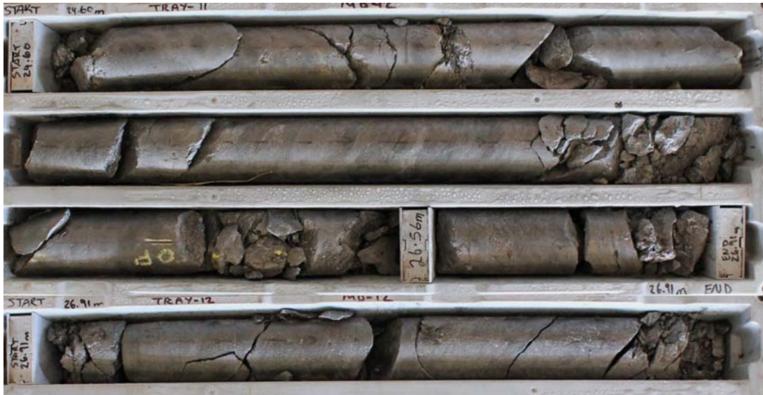
Image: HQ diamond core – Drillhole MD-12 - Central Zone of the Mount Dromedary.
