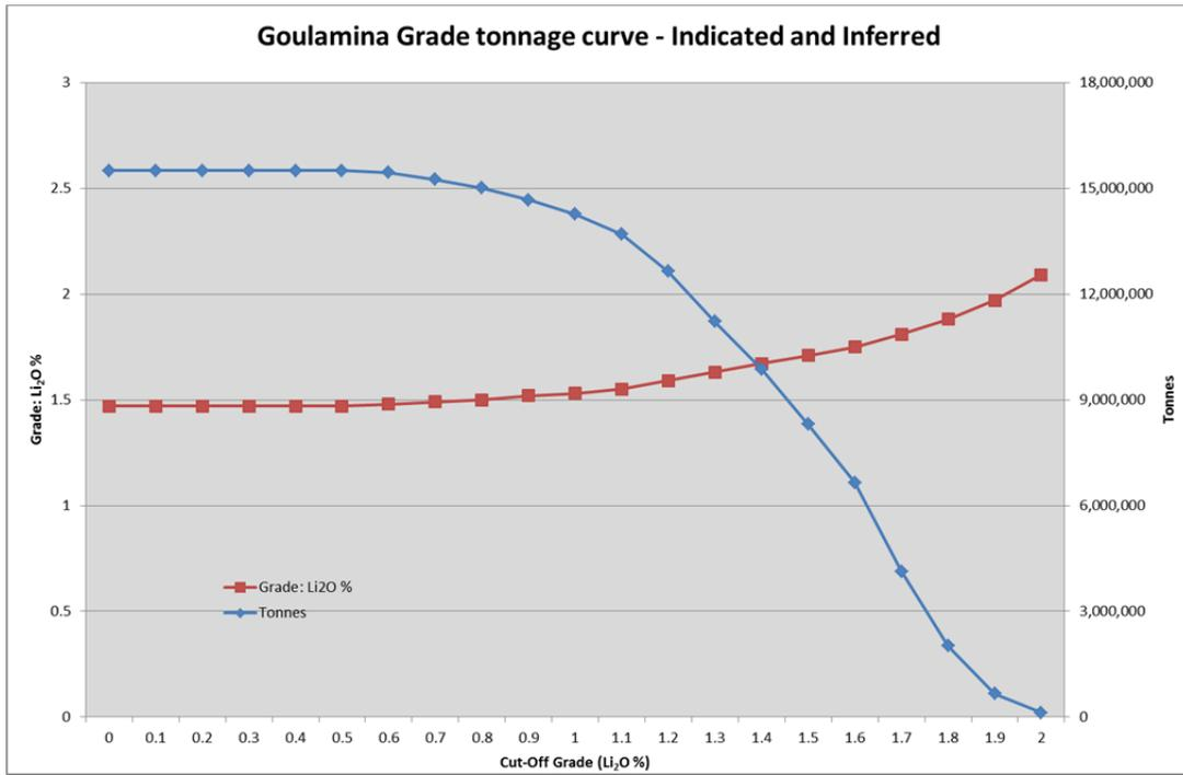
Figure 5. Goulamina Grade Tonnage curve.
