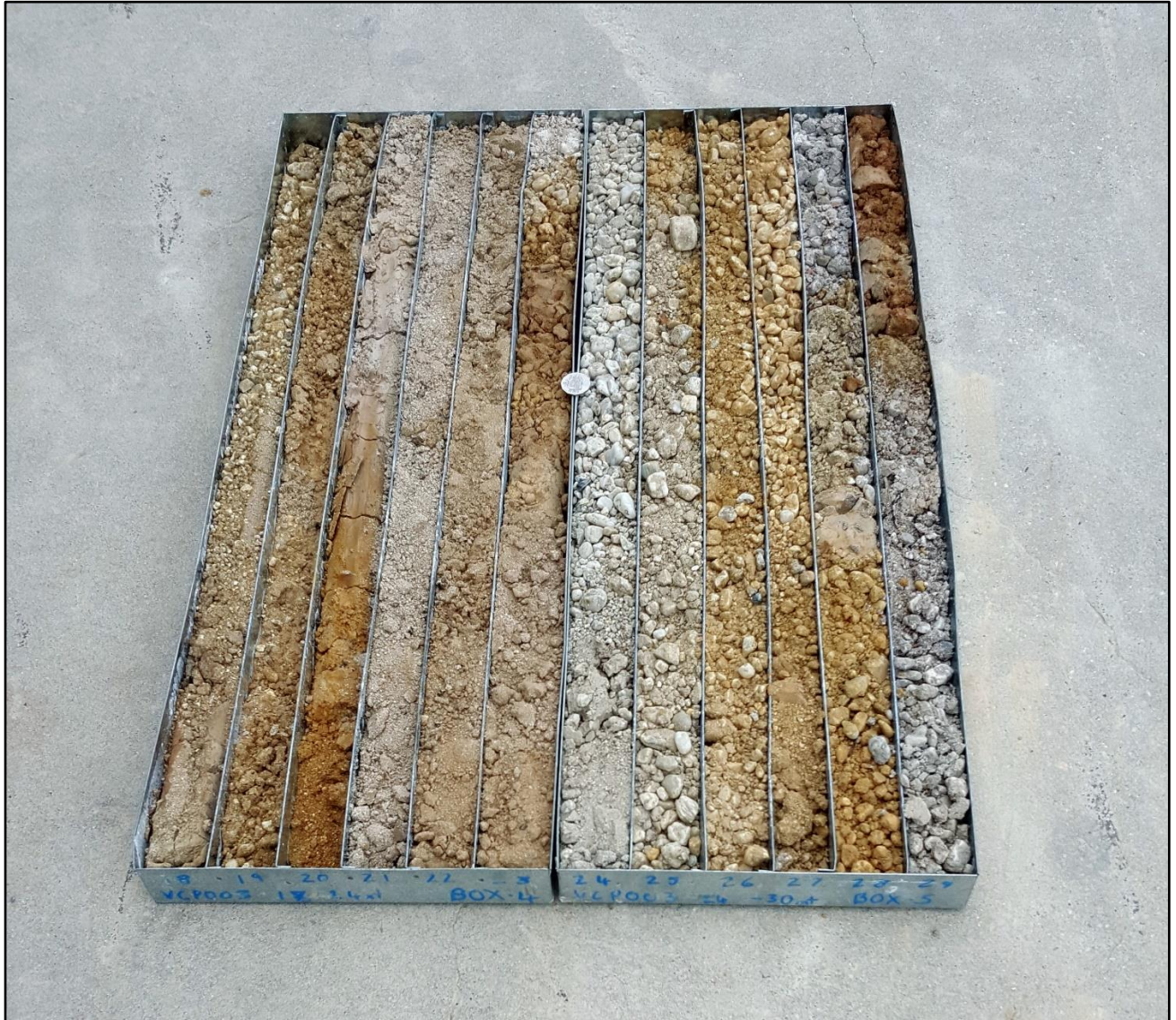
Photo 3 Sand and Quartz Aggregate Material in Core Hole VCP 3
