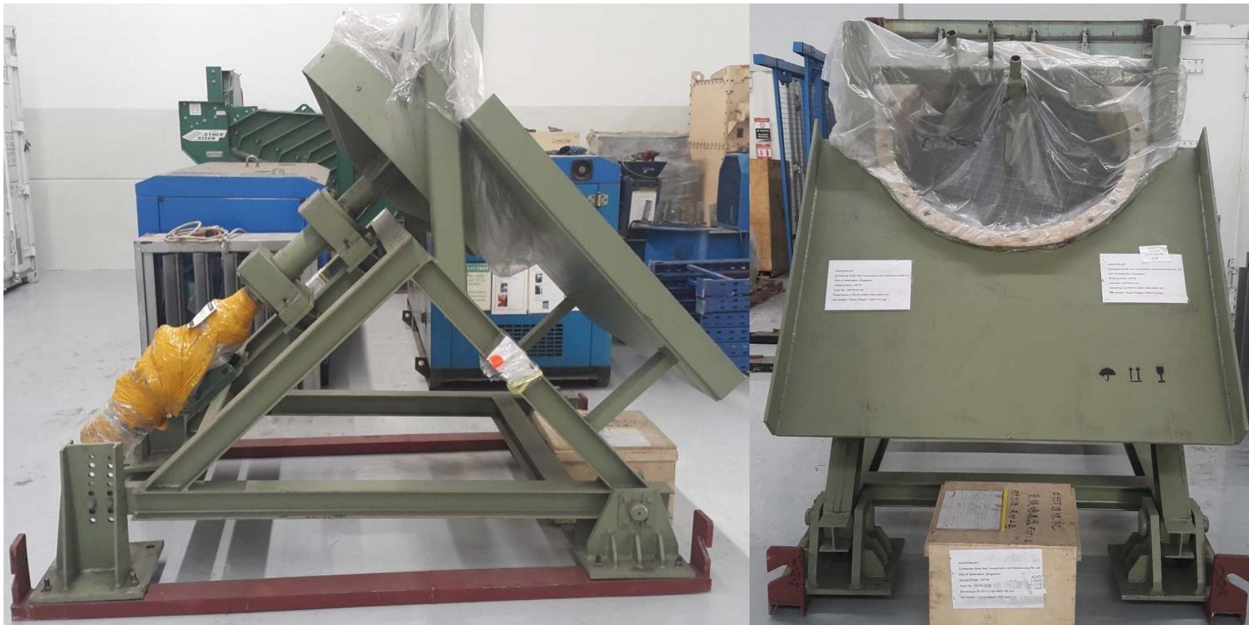
Bench Pelletizer from Jiangsu Machinery for iron sand concentrate pellet trials with GeoServices Jakarta
