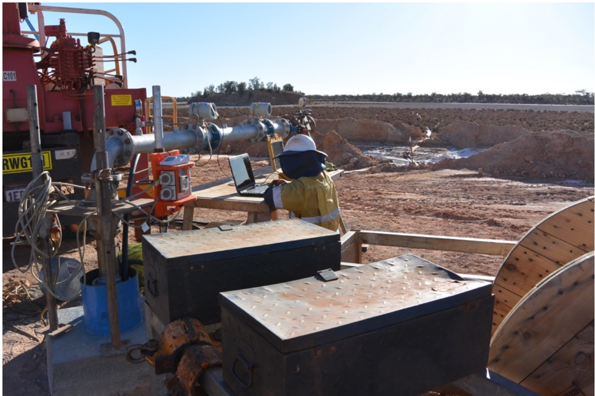
Figure 4: Test-flow pumping at TPB002 and potential evaporation pond site on the playa surface in the background
