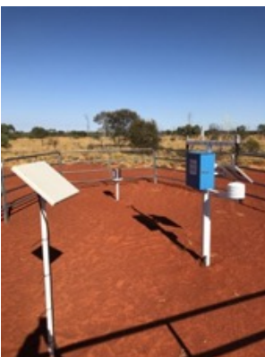
Figure 6: Weather station with installed satellite telemetry system
