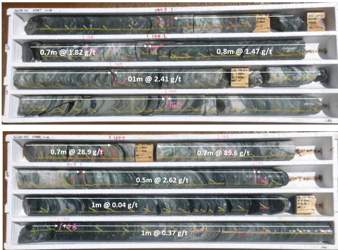
Figure 1: Diamond Core Hole 16LCDD004 showing high grade gold mineralisation up to 89.5g/t Au associated with intense quartz veining and associated sericite-siderite alteration
