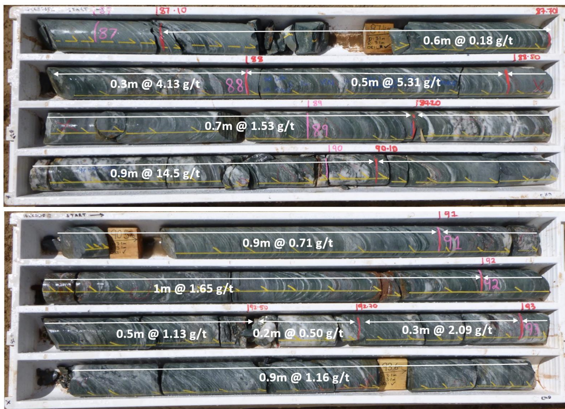
Figure 2: Diamond Core Hole 16LCDD012 showing high grade gold mineralisation up to 14.5g/t broadly correlating with quartz vein intensity
