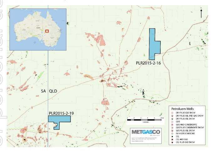
Metgasco has identified attractive plays primarily targeting the conventional Toolache Permian gas reservoir and Jurassic oil reservoirs. In addition, both blocks have the potential for unconventional gas plays in tight and reservoirs of variable quality such as the Patchawarra sands.
