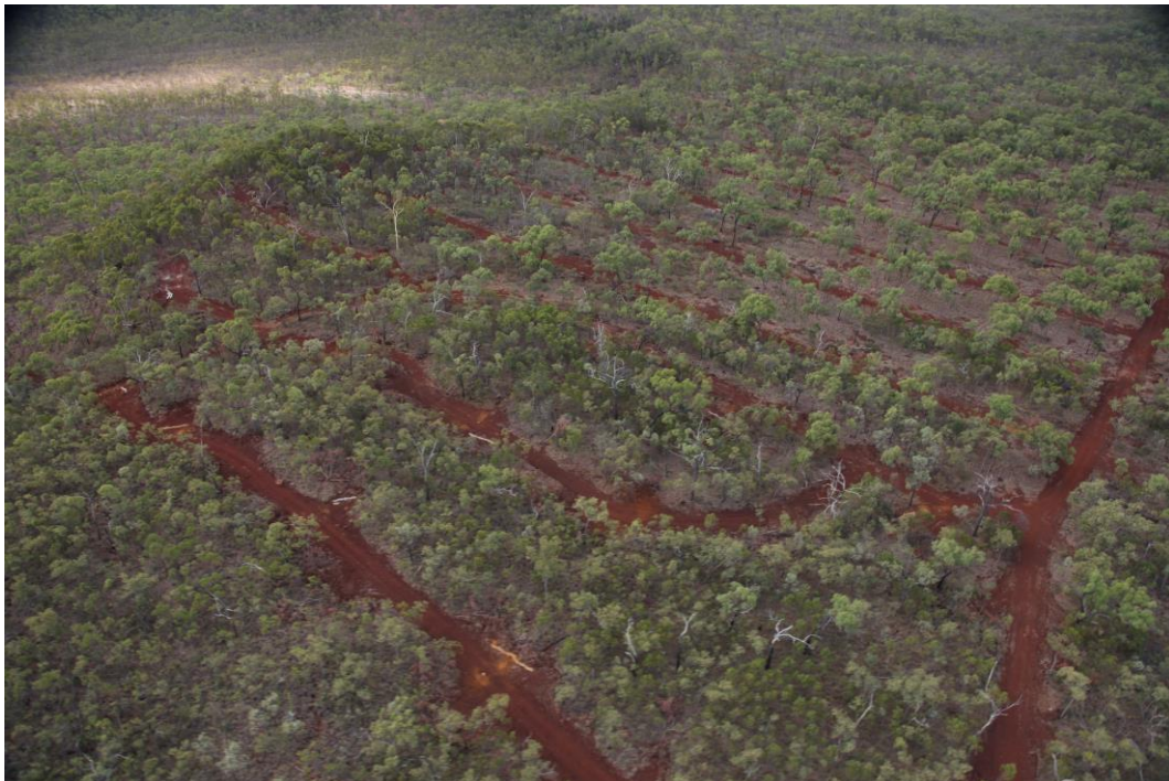
Figure 3: Aerial view of the Sconi scandium-cobalt deposit, showing the traverse lines for the upcoming resource drilling program, which is design to enable an Ore Reserve to be established.
