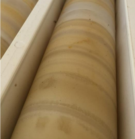
Photo: Colluli kainite core Colluli salts will be mined in solid form
