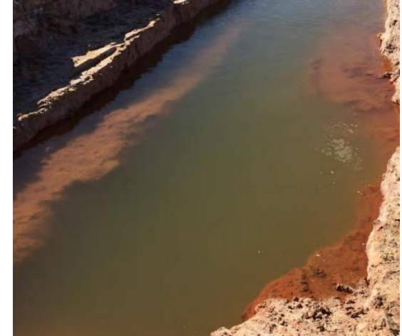
Photo: Potassium brine, Lake Wells 1 Significant evaporation required to generate harvest salt
