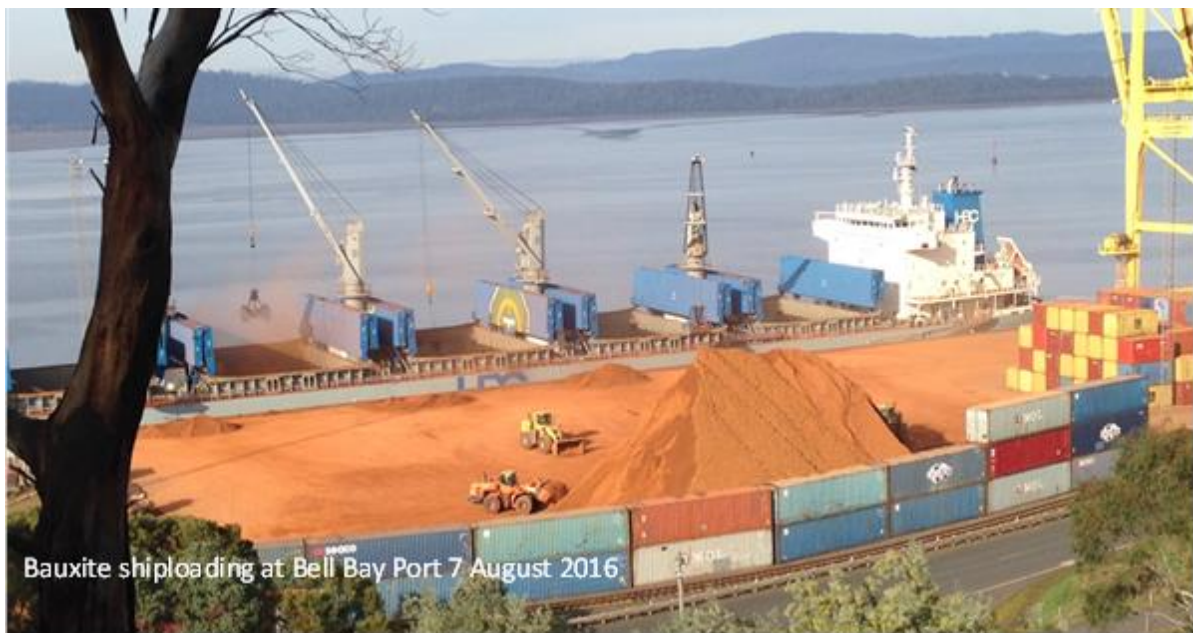
Figure 2: Bell Bay port can handle ships up to 65,000 tonnes. Loading is managed by QUBE Ports at more than 10,000 tonnes per day, achieving 20,000 tonnes per day during a loading in mid 2016
