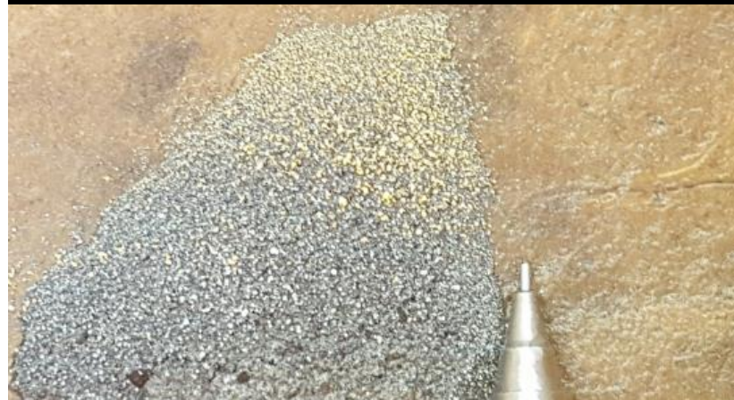
COARSE GOLD IN PANNED SAMPLE FROM 36-37 METRES IN HOLE RCDK016-37 WHICH ASSAYED >100G/T GOLD
