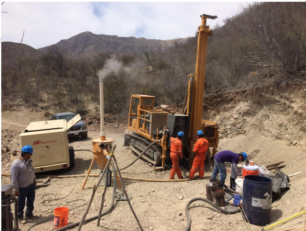
Figure 2 Reverse circulation drilling at the Agua Fria prospect, Mexico. The volcanogenic sediments that host the lithium mineralisation can be clearly seen to the right of the drill rig.
