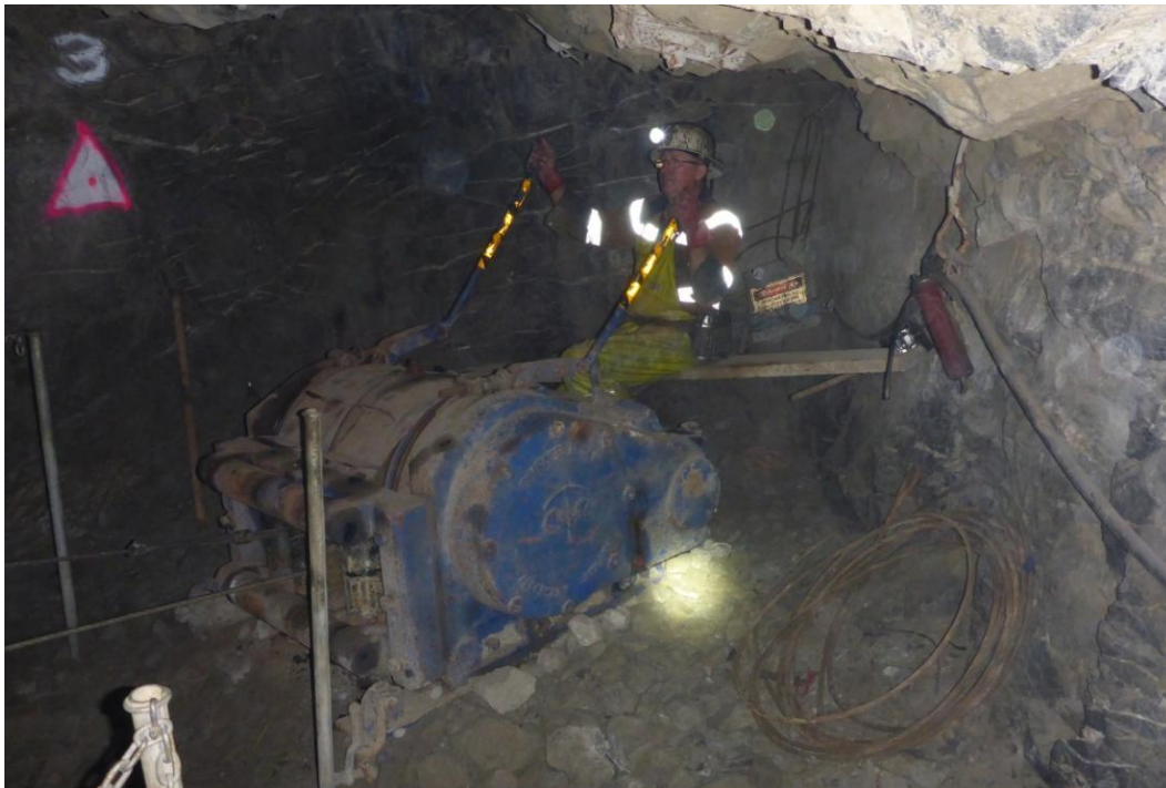
Figure 11. Air Leg Miner Mick Nolan Scraping in the 1465-8764 Air leg Stope at the A1 Mine
