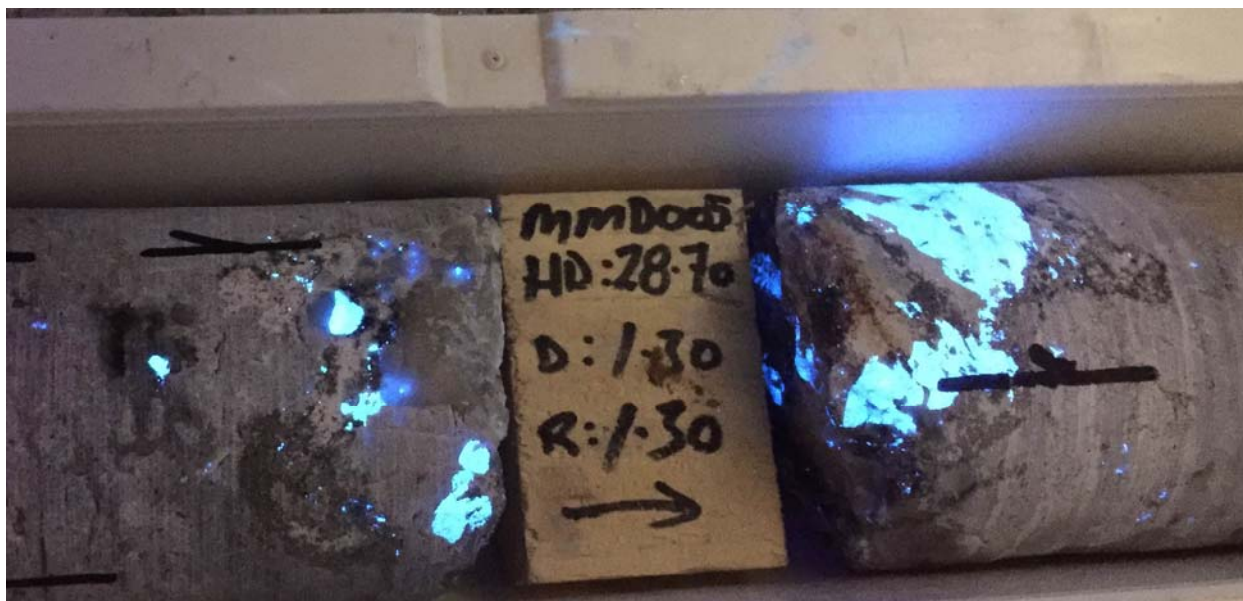
Figure 6: Diamond core from August 2016 drilling program showing course grained scheelite under UV
