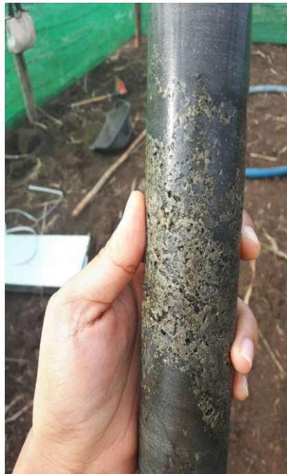
Figure 6: Vein chalcopyrite and pyrite within a broader disseminated sulphide zone in diamond drill hole 17SCDD009.
