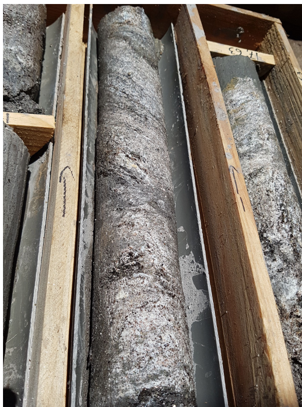
Figure 4 (above) - Cross-sectional view of the preliminary Mahefedok drilling results and Figure 5 (left)- Graphite bearing drill core from the Mahefedok drilling program.
