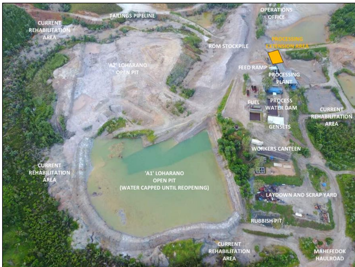
Figure 4 – Site layout showing processing extension area.
