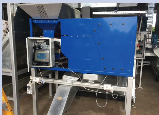
The newly installed colour sorter, which rejects any discoloured NIS, reduces the requirement for manual sorting
