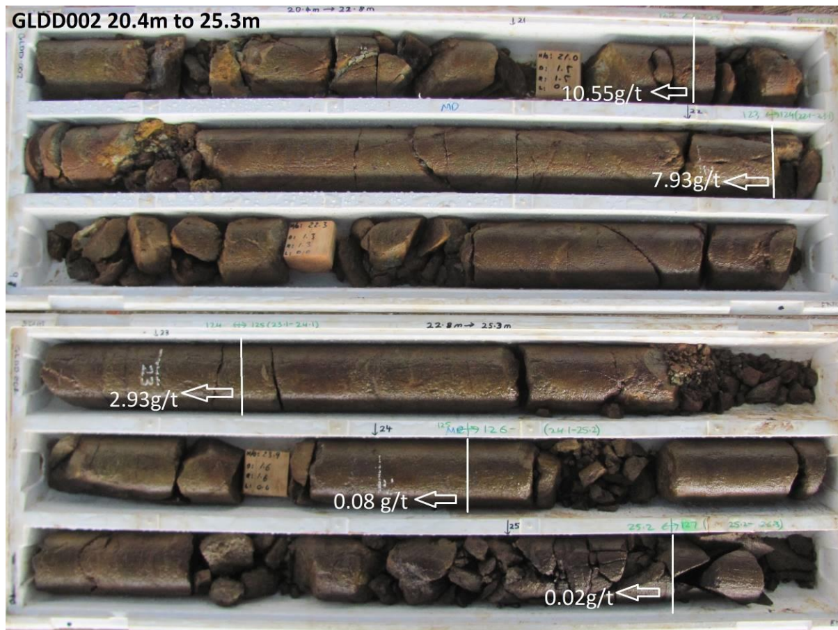
Photo 2: GLD002 in the 20.4m to 25.3m interval. Weathered dolerite with narrow quartz veins.
