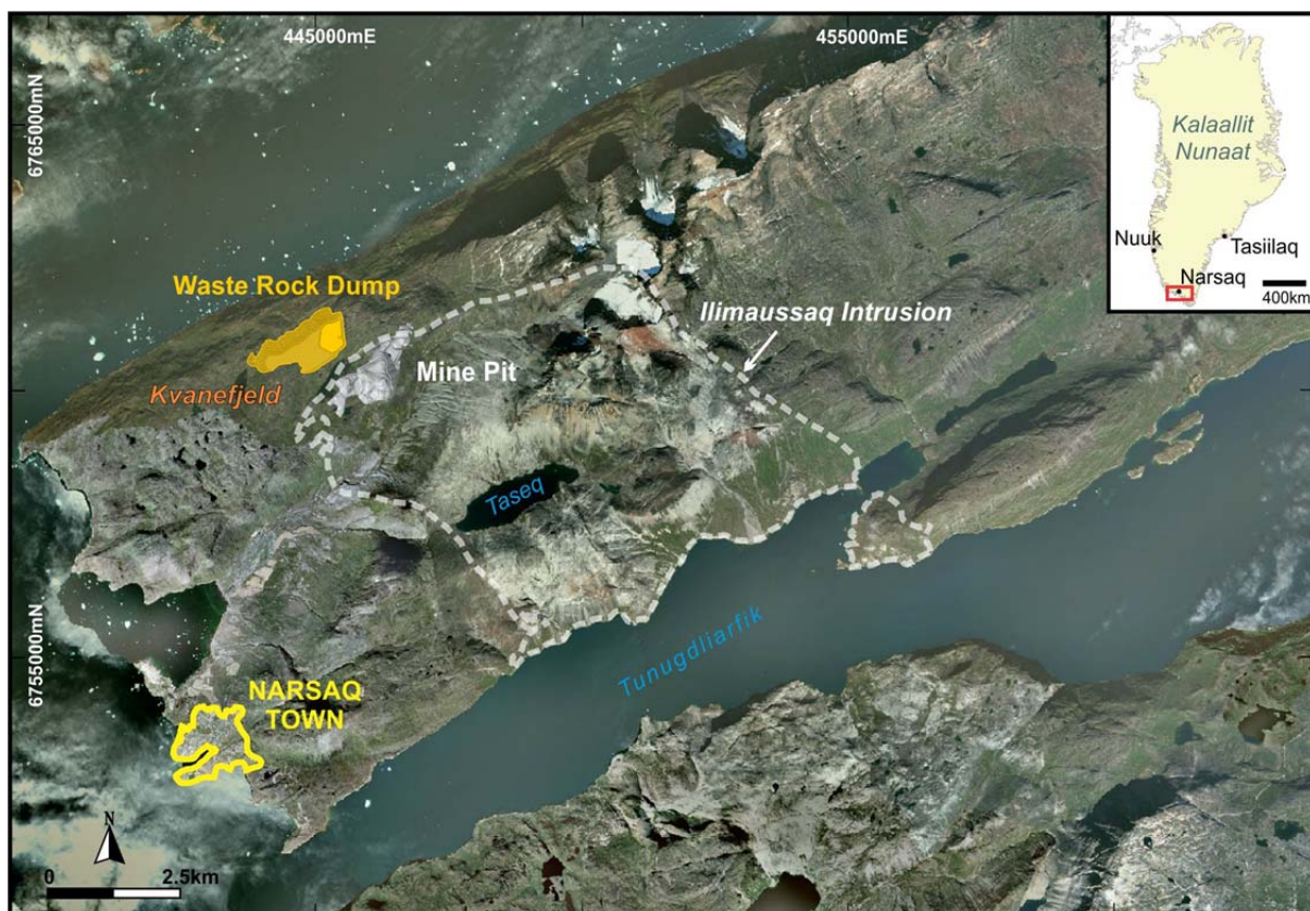
Figure 1. Overview of the Narsaq Peninsula, southern Greenland, and the Kvanefjeld Project area. Unmineralised (waste) rock is to be deposited in contoured mounds (dumps), located to the northwest of the mine area. The waste rock dumps will not be visible from the town of Narsaq, and will consist of common rock types that are widely present throughout the Project area.
