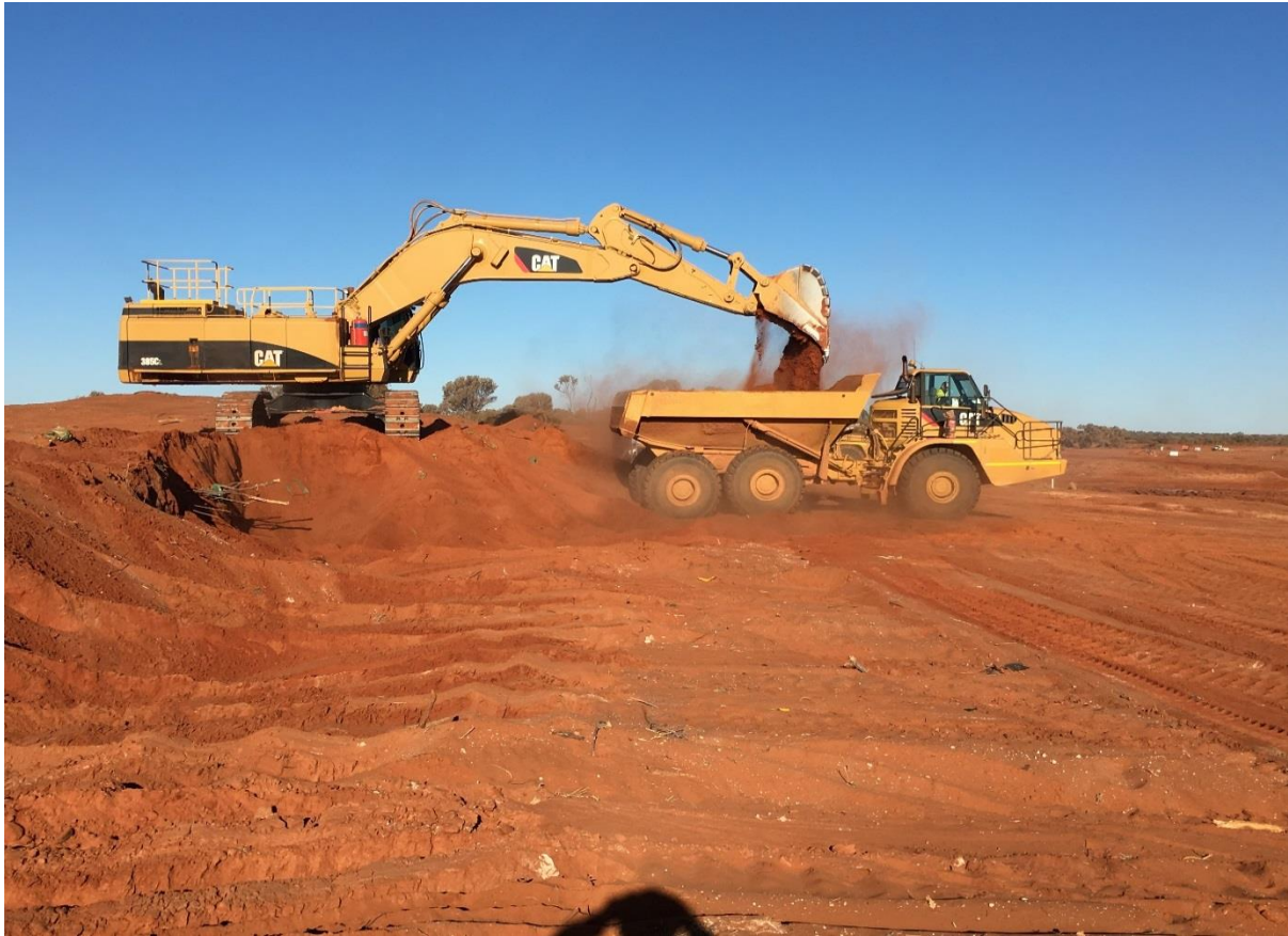
Figure 1: Overburden Mining in the North Pit
