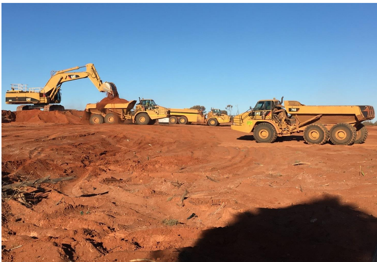
Figure 4: Overburden Mining in the North Pit
