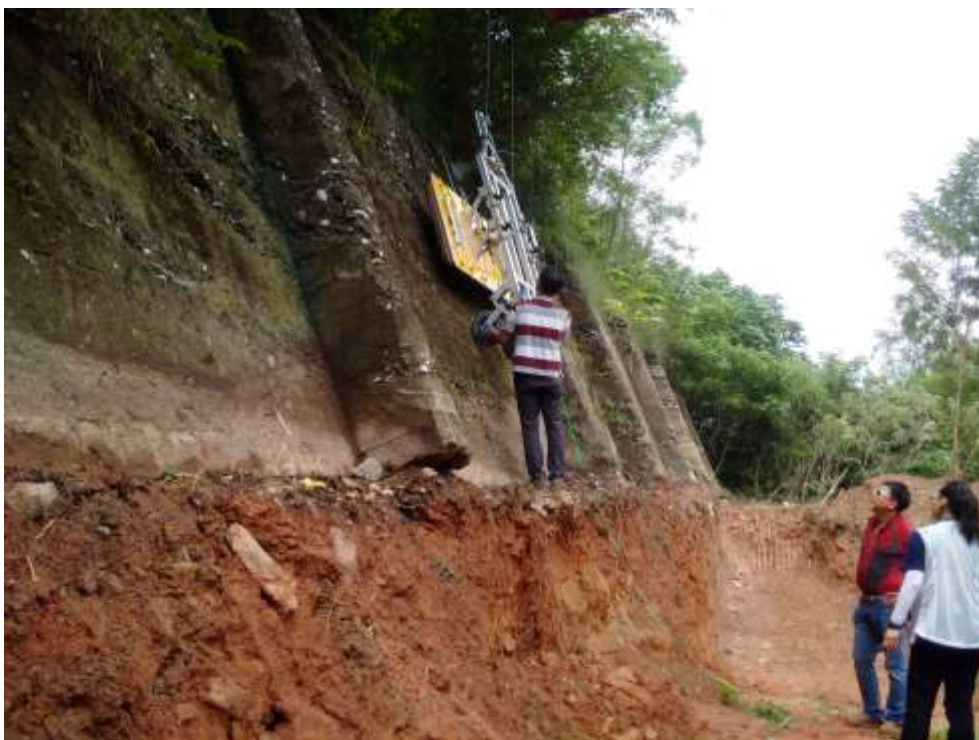
Photo 5. Ground Penetrating Radar being used to locate main adit entrance
