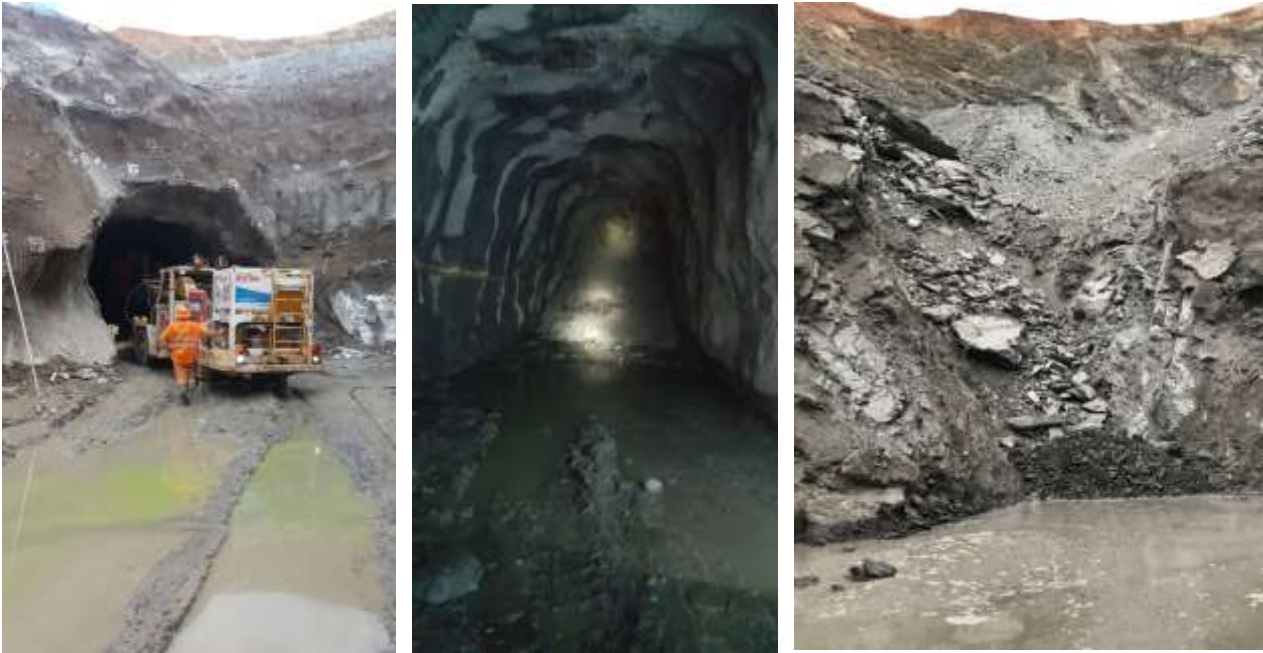
Photo 2-4: Cannon Adit - portal, development drive with first firing and stope blast.
