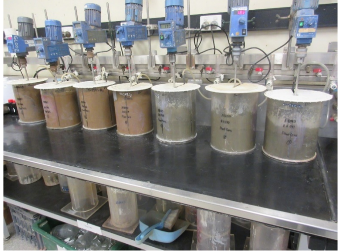
Figure 2 & 3. Sample preparation and open vat testwork at ALS Laboratories Perth in preparation for demonstration plant metallurgical test work
