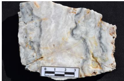
Polyphased hydraulic vein breccia & colloform-banded vein comprised of white mesocrystalline quartz with grey-black sulfidic inter-bands and wispy fills
