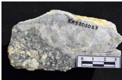
Polyphased hydraulic vein breccia with rip-up vein fragments and a central black sulfidic band comprised of fine-grained pyrite & sulfosalts
