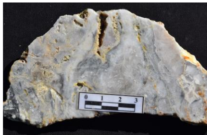
Polyphased, crudely banded mesocrystalline grey-white quartz vein with localised ghosted quartz pseudomorphs after bladed calcite & wisps of bluish-grey sulfides & sulfosalts
