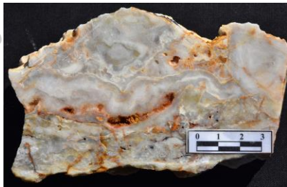
15 cm wide polyphased vein float, comprised of hydraulic rip-up breccias and crude mesocrystalline to chalcidonic quartz colloform band development.
