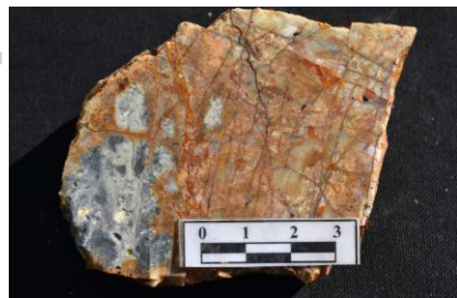
Hydraulic quartz vein and rhyolite host rock breccia, pervasively flooded by mesocrystalline quartz and fine-grained pyrite. Highly oxidised with ubiquitous limonite after pyrite
