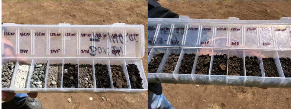
Figure 3 – Boxes of Chips of BER223-17 RC Drilling. Intervals of Zn > 3%
