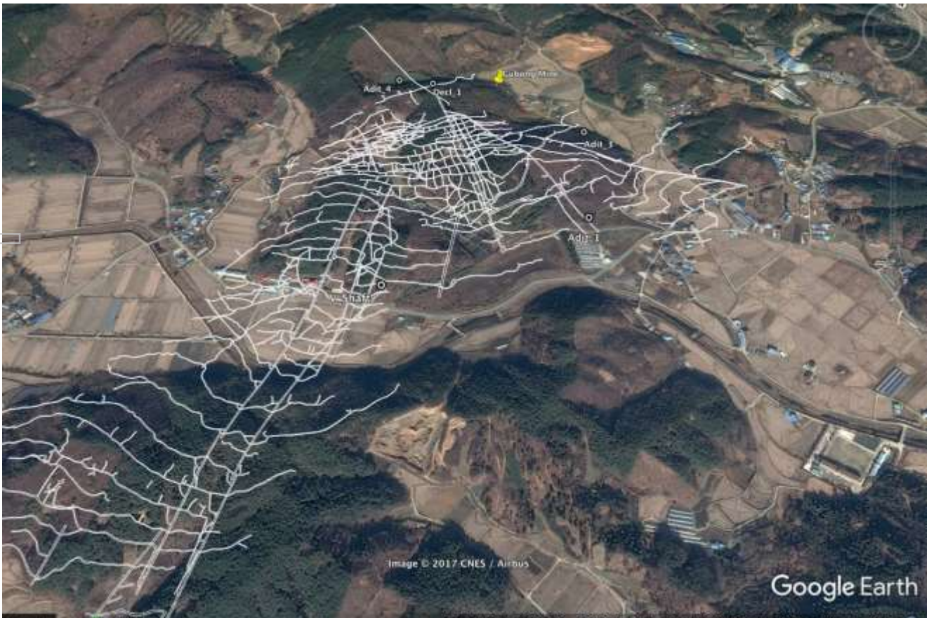
Figure 2: Google Earth image draped over the historical underground mine workings.
