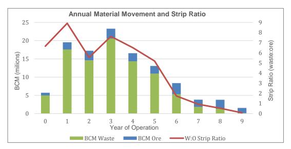
The single open pit will be mined in two stages to assist in reducing total earthmoving production requirements and in particular the first two years of operation. Additional detailed scheduling will be required to further optimise material movement and manage the estimated 20 to 25% of Potentially Acid Forming (PAF) waste material contained within the pit.
