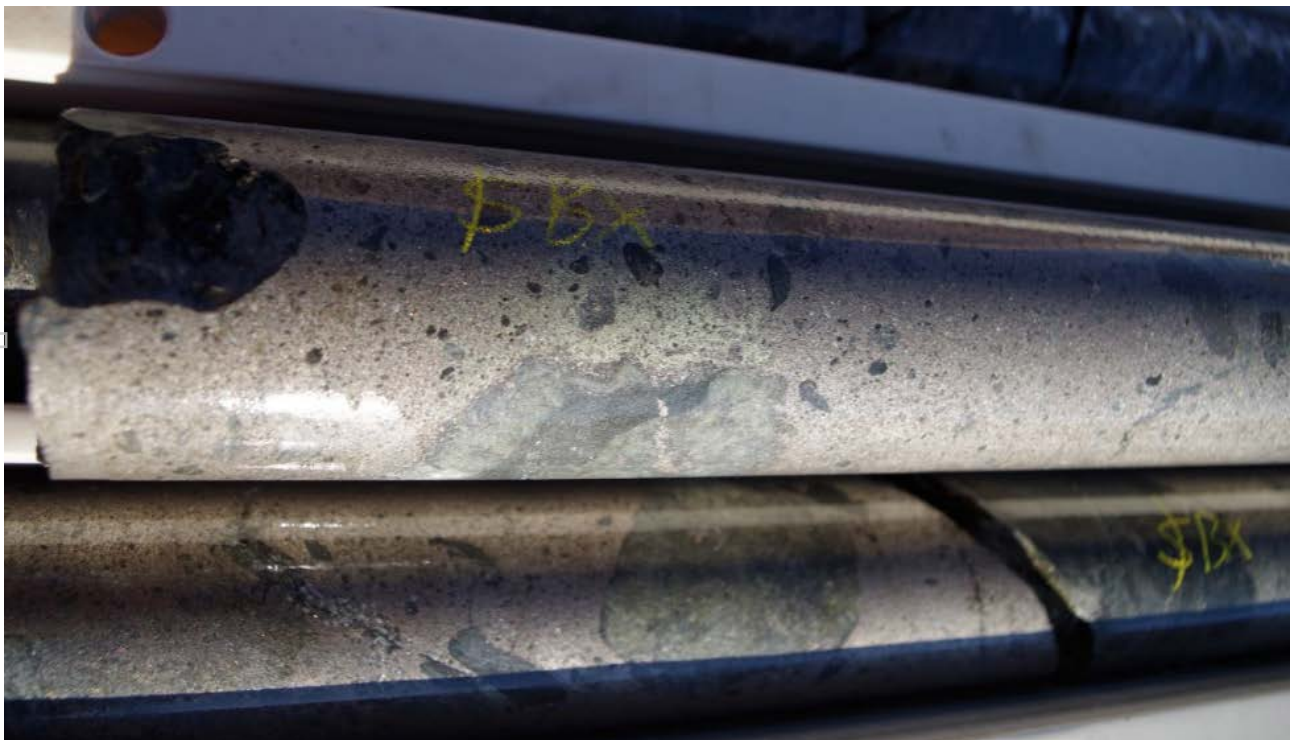
Figure 5: Grapple NQ core with pyrrhotite-chalcopyrite breccia sulphides in the lower mineralised zone of 17GRDD005
