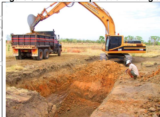
Exploration pitting at Blina using an excavator
