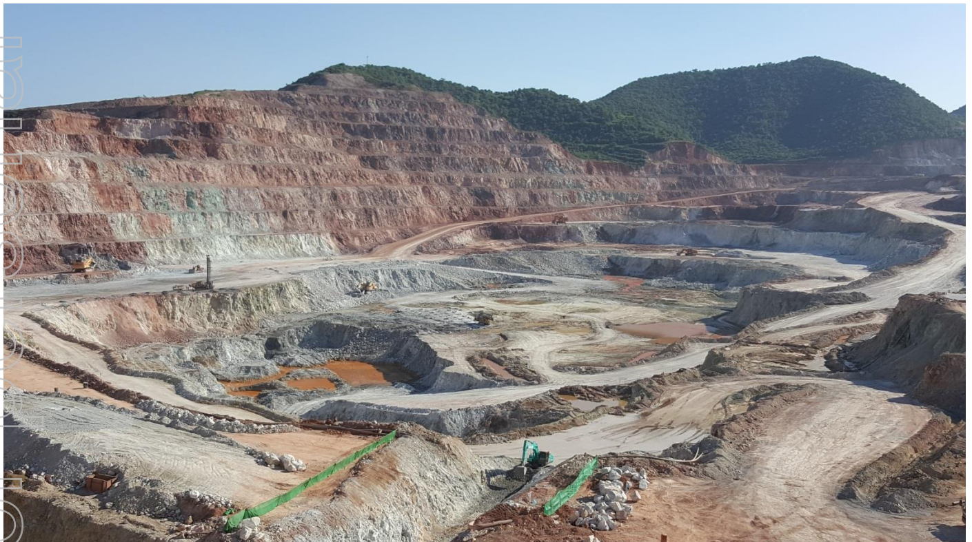
One of Wanbao Mining Limited's copper mines in Myanmar that is expected to produce over 100,000 tonnes of cathode copper next year from an extremely efficient bacterial sulphide leaching operation.
