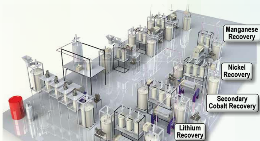
Figure 7: Schematic of Li-ion Battery Recycling Pilot Plant under construction
