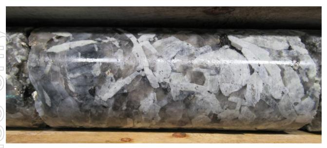
Figure 2: Spodumene crystals in hole 17-32 at 34.5 metres.
