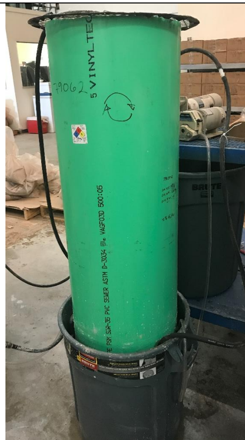
Short (1.5m) column containing 150kg sample that was leached for a total of 41 days with recoveries of 92% lithium and 89% boron.
