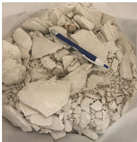
Sample after column leach test 90% of Li and B removed Integrity of the rock remains Very favourable characteristics for heap leaching
