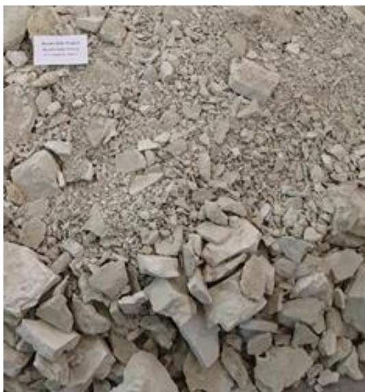
Sample before column leach test Lightly crushed to minus 150mm Coarse material with low percentage of fines
