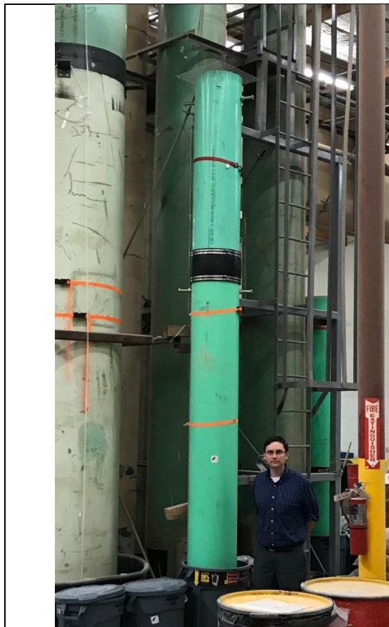
Tall (4.4m) column containing 495kg sample that was leached for a total of 164 days with recoveries of 89% lithium and 89% boron.
