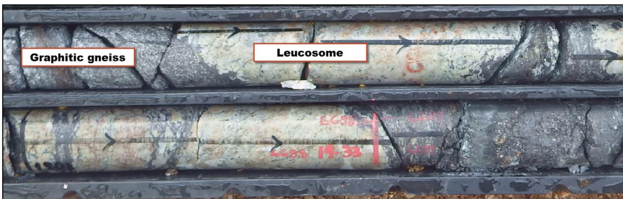
Figure 6: Detail showing graphitic gneiss and leucosome of granitic composition in IVD041
