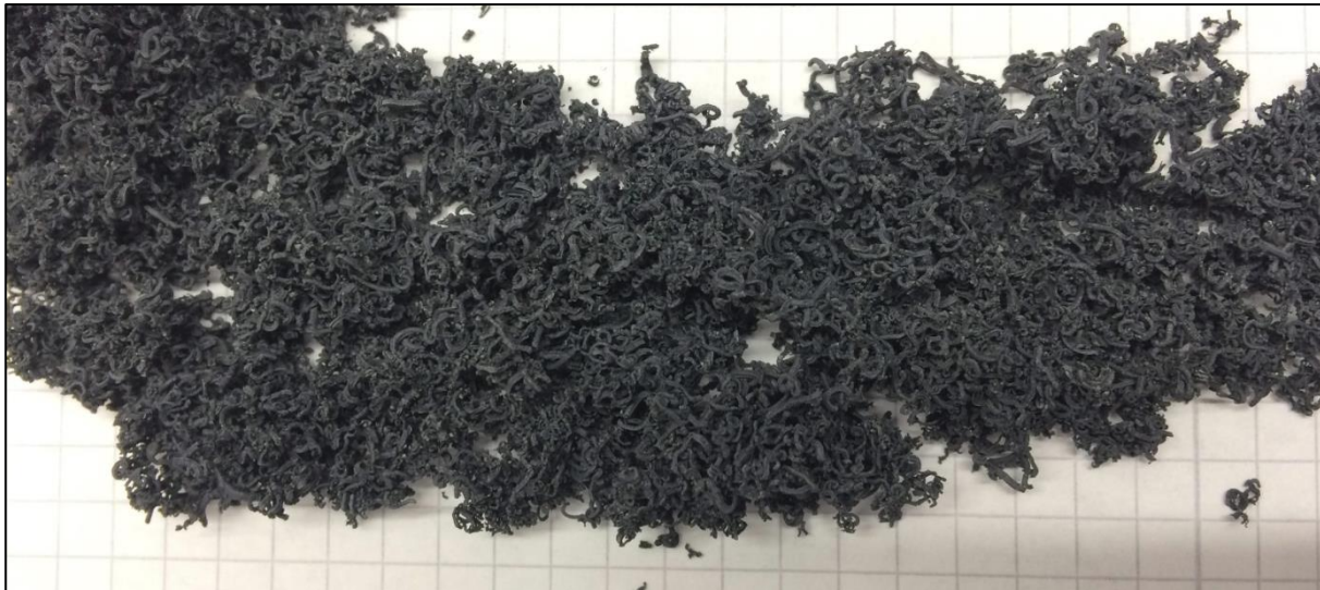
Figure 25: Ancuabe +50 mesh concentrate converted to expandable graphite and exfoliated
