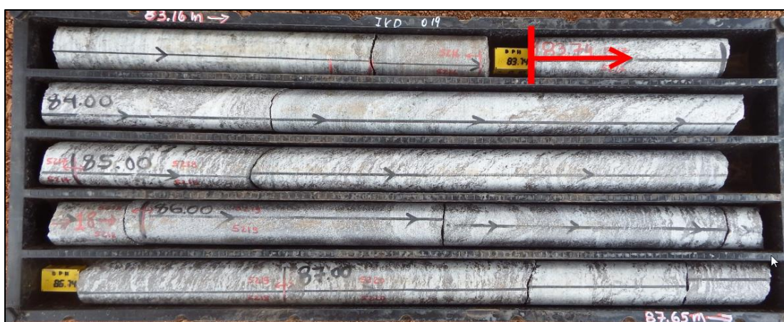
Figure 6: Graphitic gneiss (~ 6% TGC) between 83.74–87.65 m downhole in IVD019. Mineralisation zone 1
