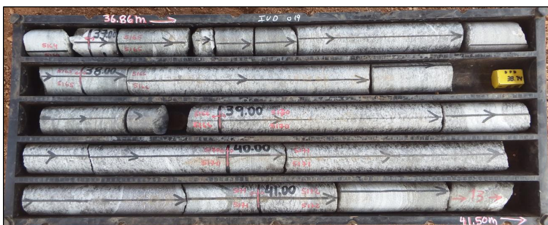
Figure 5: Graphitic gneiss (~ 7% TGC) between 36.86–41.5 m downhole in IVD019. Mineralisation zone 2
