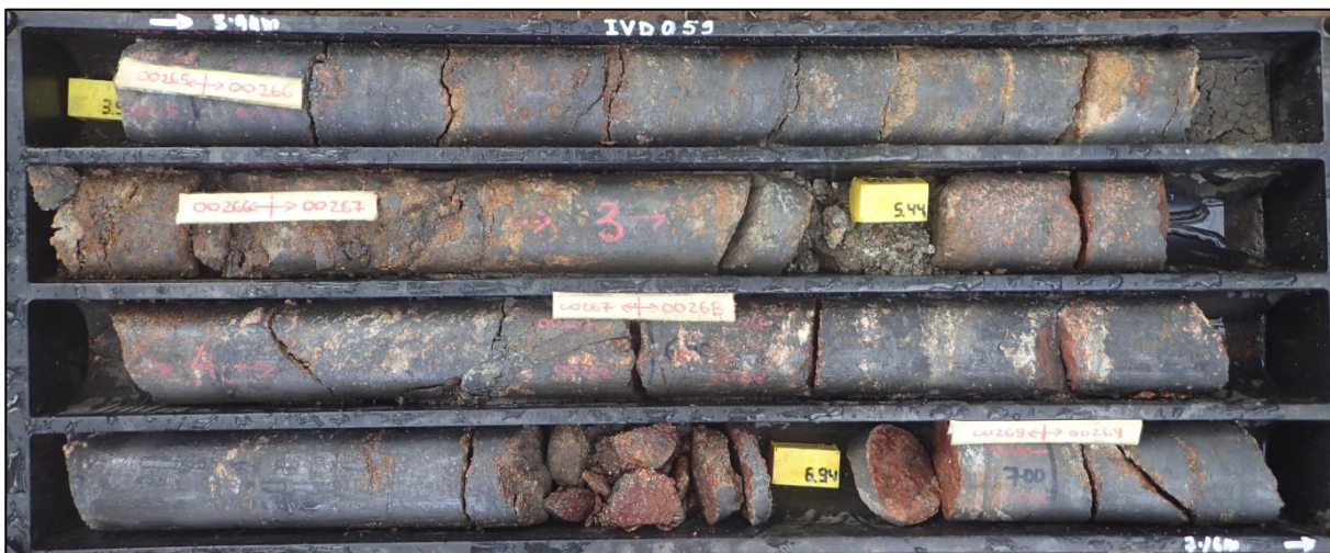
Figure 4: Oxidised graphite gneiss between 3.94 m and 7.16 m in IVD059 (~ 10% TGC)
