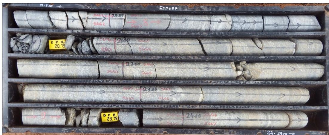
Figure 4: Graphitic gneiss (~ 7% TGC) between 19.7–24.4 m downhole in IVD027. Mineralisation zone 15
