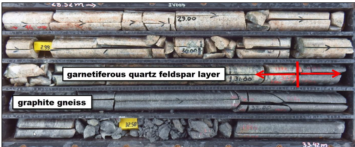
Figure 7: Garnetiferous quartzo-feldspathic layer and graphitic gneiss in IVD014. Mineralisation zone 2
