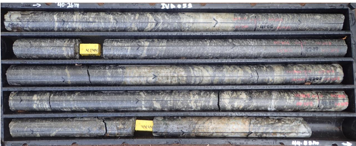
Figure 5: Fresh graphitic gneiss from 40.26 m to 44.85 m in IVD059 (~ 9% TGC)
