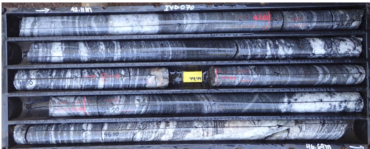
Figure 7: Amphibole and garnet bearing gneisses in the footwall of IVD070
