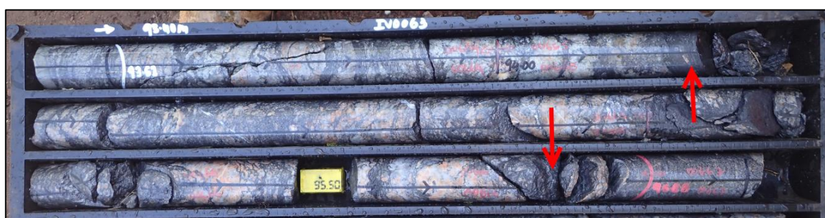
Figure 9: Brecciated and mylonitised graphite gneiss with graphitic slickensides in Mineralisation Zone 2 at approximately 93 to 96 m depth in IVD063
