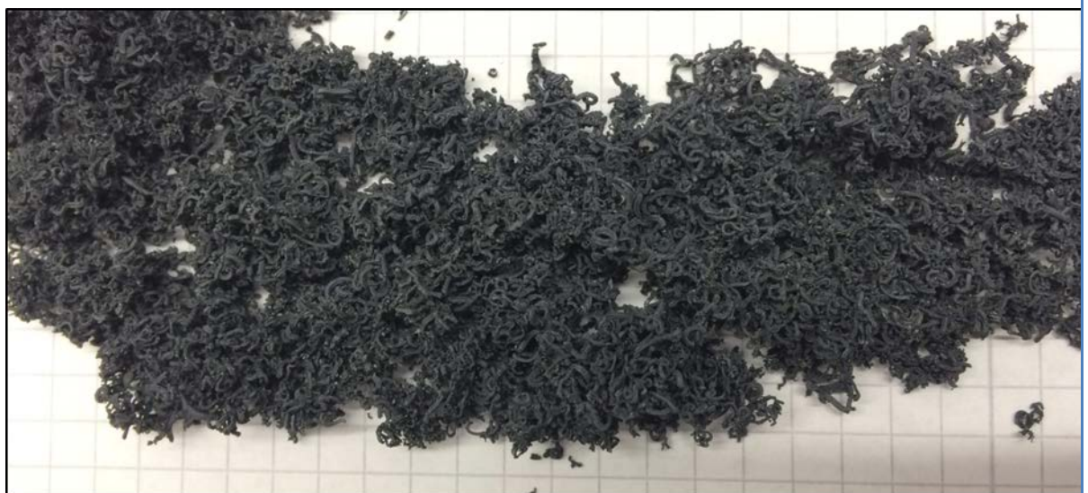
Figure 11 Ancuabe +50 mesh concentrate converted to expandable graphite and exfoliated to >320 mL/g
