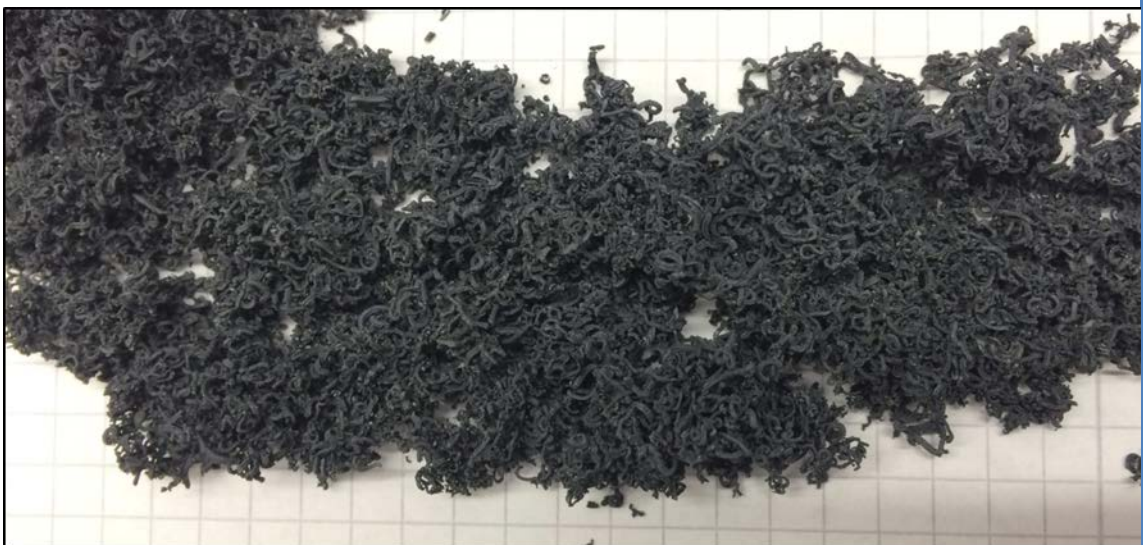
Figure 13 Ancuabe +50 mesh concentrate converted to expandable graphite and exfoliated to >320 mL/g
