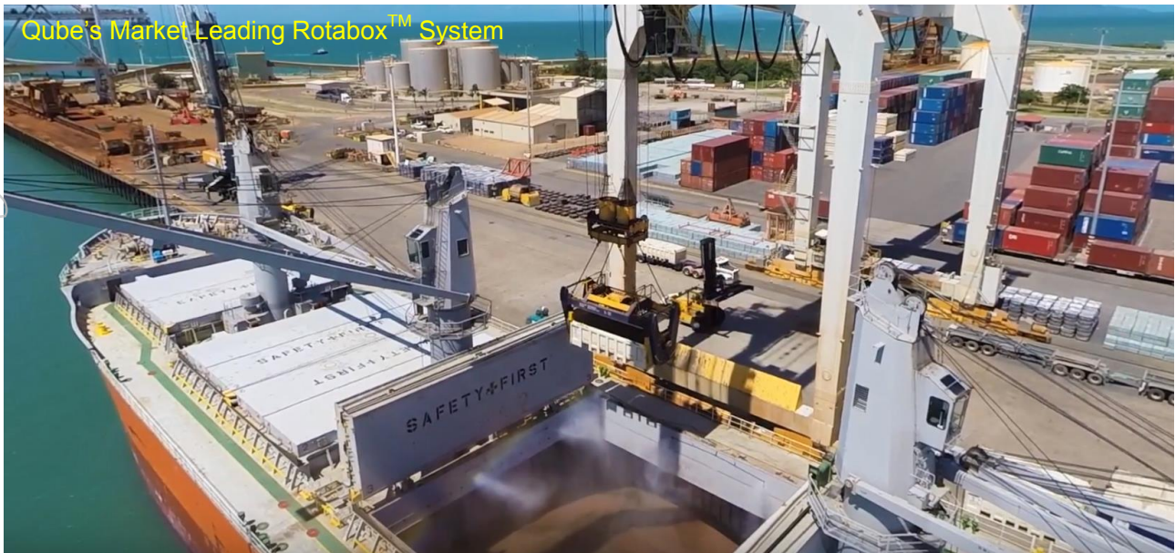
FIGURE 25: Mineral concentrate being loaded at the Port of Townsville using Qube's Rotabox™ system.
