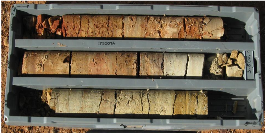
FIGURE 18: PQ diamond core from mini-composite.
