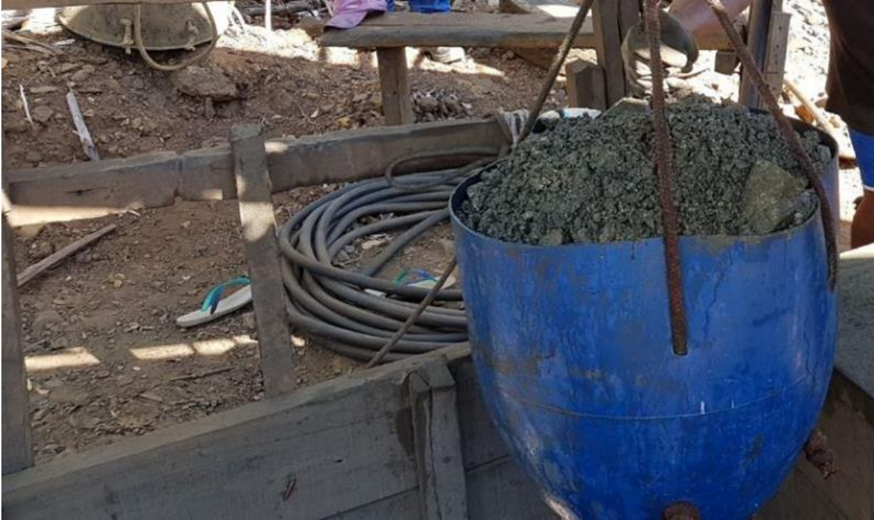
Figure 4: Massive chalcopyrite hoisted from a small 20m deep artisanal shaft (eastern side of Pantera)
