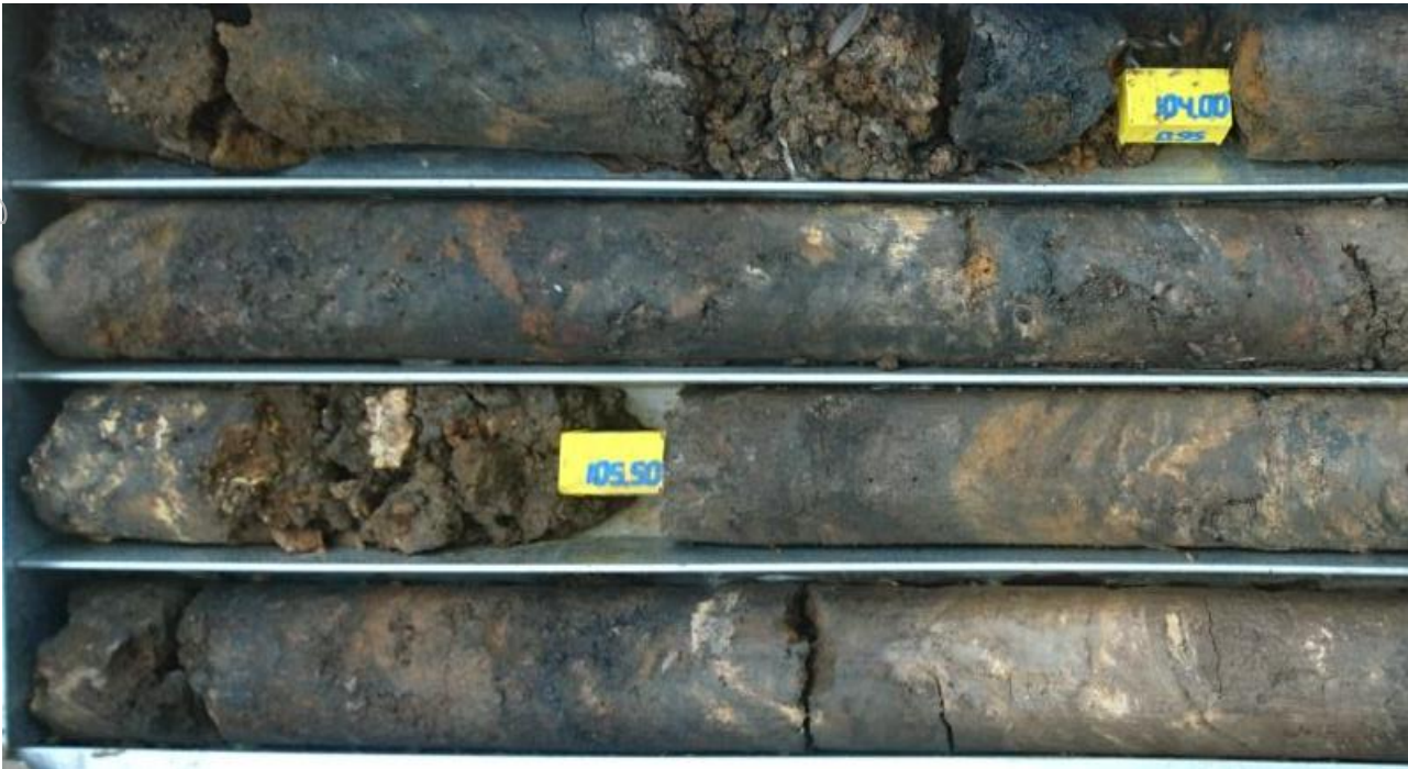
Figure 6: Heterogenite mineralisation in drill core from DMON7_DD01.
