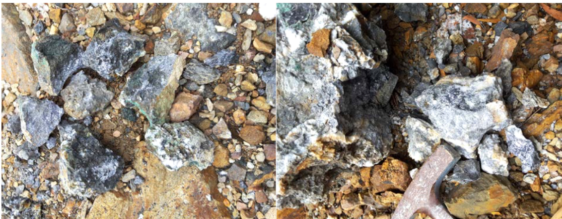
Figure 2 – Photos of rock chip samples ARDQ03 (LHS) and ARDQ04 (RHS) showing massive galena and minor chalcopyrite hosted by carbonate and shale
