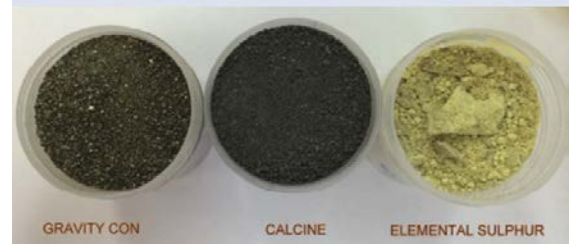
Above: Laboratory-scale furnace & elemental sulphur condenser. Below: Photos of the feed concentrate, residual calcine and collected elemental sulphur.
