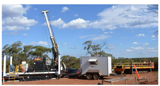
FIGURE 4 – DIAMOND RIG DRILLING AT ROTHSAY
