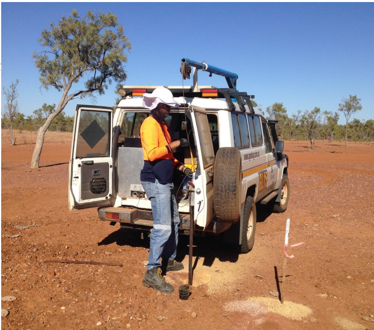
CAPTION: Down-hole geophysical gamma logging at Ardmore.
