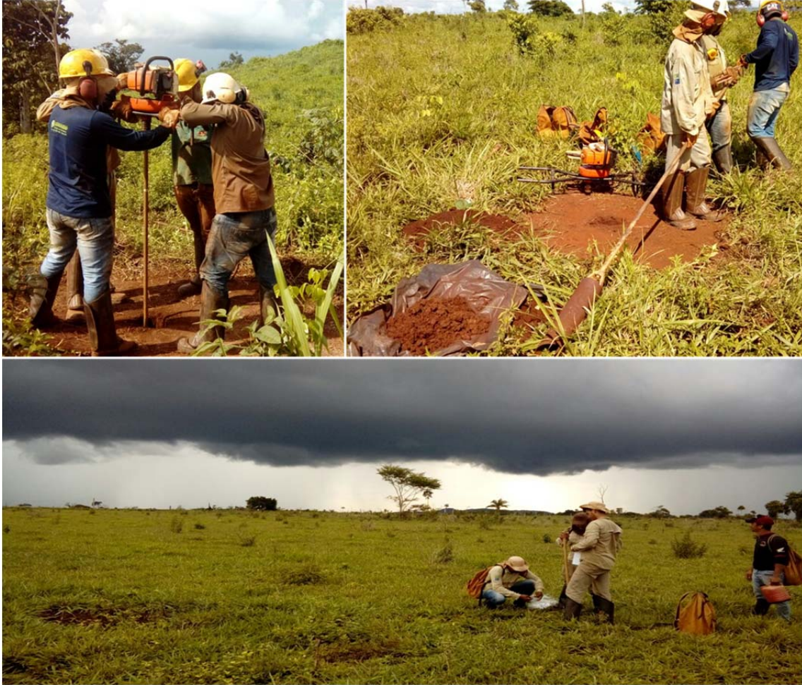
Figure 4 – Photos of the auger drilling at the Itapitanga Ni-Co Project; Four man hand held auger (top left), removing the sample from auger bit (top right), working to beat the afternoon rain (bottom).
